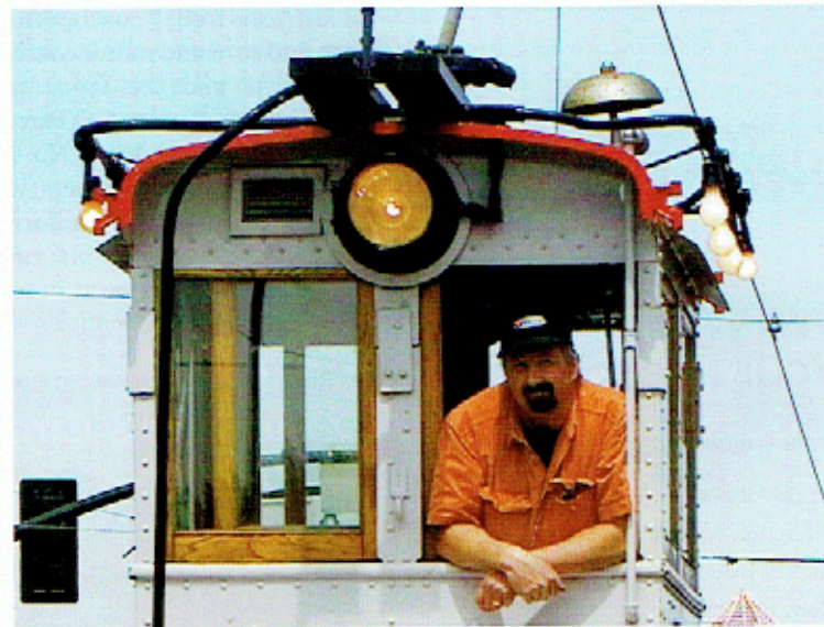
Karl in the cab of 1916 Muni work car C-1, which he piloted many times on its trips to check alignment of newly laid track and switches. SFMTA photo.
