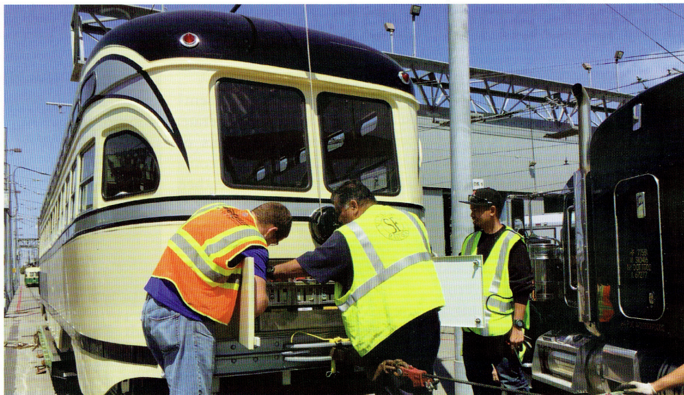
IT'S ALIVE! —The Muni maintenance team, captained by Manny Enriquez (center) connect the battery leads to energize Car 1056 after unloading.
