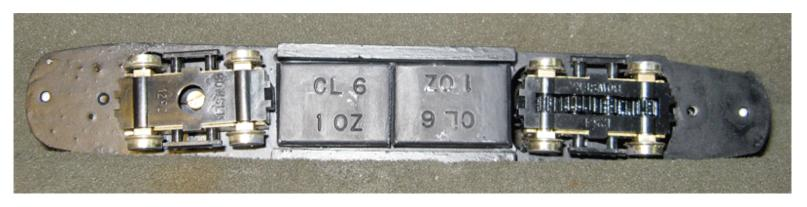
The weight of the car was not the only issue modelers may face when trying to operate this car on tight curves. Another concern involved the combination of the lack of cutouts in the skirts on the car with the longer than normal truck center-to-center wheelbase and the fatter than than prototypical RP-25 wheels, which could restrict truck swivel. This could result in the car not be able to operate on small radius curves.
