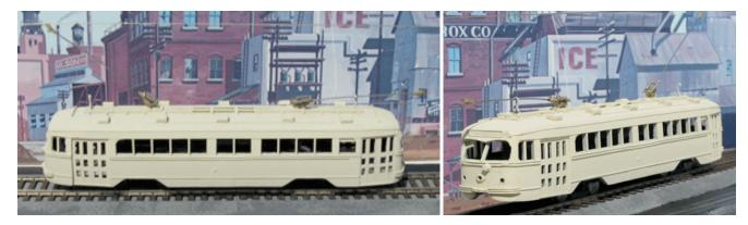
We gathered up portions of the Custom Traxx CN-1040 and CN-178 decals. Using portions of both of these, we could complete the finishing of our first car. We will also match the green and cream with the Bowser F-line PCC #1050 and we should be in great shape. As we found out, Floquil 183, Reading Green was a close enough match for the Muni green and of course Floquil 85, Antique White is our standard cream color.
