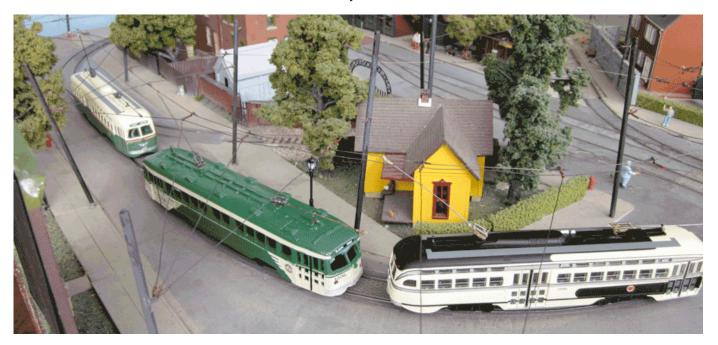
This "Torpedo" model is equipped with the Bowser drive used as a test bed for the Bowser F-line PCC cars. In addition to the Bowser 79 motor, the unit is equipped with a Stewart flywheel and drive line, wheels with the super resilient wheel faces now used on the 12600 series of Bowser PCC cars and the Bowser 12600 PCC Form 11 Trolley pole and pivot. Concluding this updated article are some recent photos taken on the Southern California Traction Club test track.
