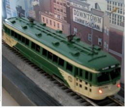
As we have discovered, this shell can be used as a beginning to get a good model of San Francisco series 1016-1015 "Torpedo" PCC. If the modeler is knowledgeable about the prototype, can use a milling machine and is willing to put in a little effort, he or she can eventually get a superior model.
