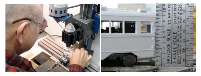
1. We cut the rear of each side to allow installation of the double rear doors. John McWhirter is pictured in the above left photo using his milling machine. We did this to both shells during the same work session. The next photo shows the shell cut for installation of the rear door
