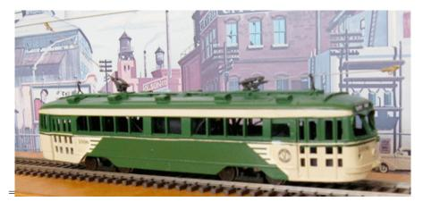
We eventually installed our Train Control Systems M1 decoder along with Miniatronics 1.2mm diameter 1.5 volt lamps on both ends of the car. There are two red taillights and one headlight on each end of the car and they are reversible and controlled by F0. The two taillights were installed in parallel but in series with a 220 ohm resistor while each headlight was installed in series with a 560 ohm resistor.
