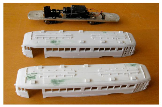
In the previous photo, at the top is the Bowser F-line mechanism mounted on the Custom Traxx 125164 pewter floor. In the middle and bottom are the two shells that have had three of the four vents removed along with the removal of both original trolley pole bases.
