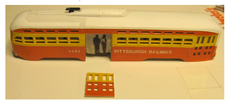
b. After stripping the paint from the door and a little filing, it fit perfectly. We actually preferred the Bachmann doors to those we used on the first car. We added the same .010" x .030" styrene to the base of the door for the bottom step.
