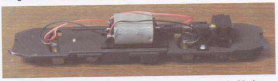
4. Install Motor on its brackets using 2-56 screws provided with the Bowser drive. Solder the wires to the motor (separate them first if they are 2-conductor, like we used) and fold down as shown to a low profile. Assemble (if necessary) and install the driveshaft. Cut the metal rod provided for it to about 11/16" (15mm) long. Lubricate bearings and gears and give it a test-run.
