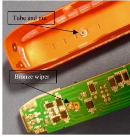
If you don't have a MTS PCC pole the same result can be accomplished by filing flat the head of a 2-56 screw and drilling the appropriate size hole for your poles lengthwise through the screw. This will produce a very workable pole bushing. If a non-PCC pole is used, be certain that the base sits high enough that the swing does not foul the pole shroud and cause dewirement.
